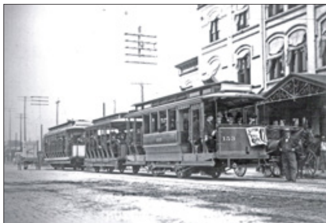
The open car was used during the hot humid Houston summers to catch a breeze through the car. Shades could be pulled down to keep out rain if necessary. The number of passengers indicated the importance of streetcars to Houston transportation at the time.
