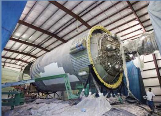
**Multiple layers of the rocket’s exterior paint were removed using ultra-high pressure water jets.**
