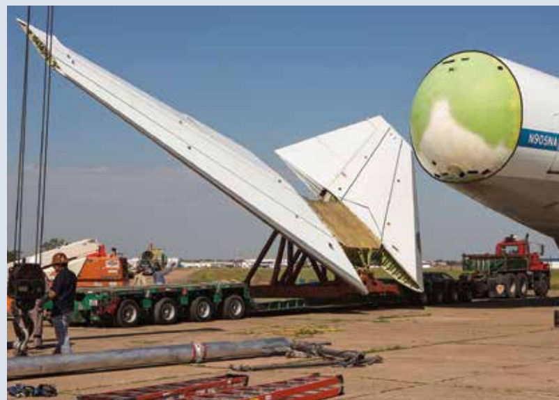
The horizontal stabilizer and elevators were removed from the rear of the 747, exposing a portion of the fuselage that helps maintain cabin pressure. Also removed were the specially made vertical stabilizers placed at each end of the horizontal stabilizer of NASA 905 (and her sister carrier NASA 911) to enhance directional stability. 7
