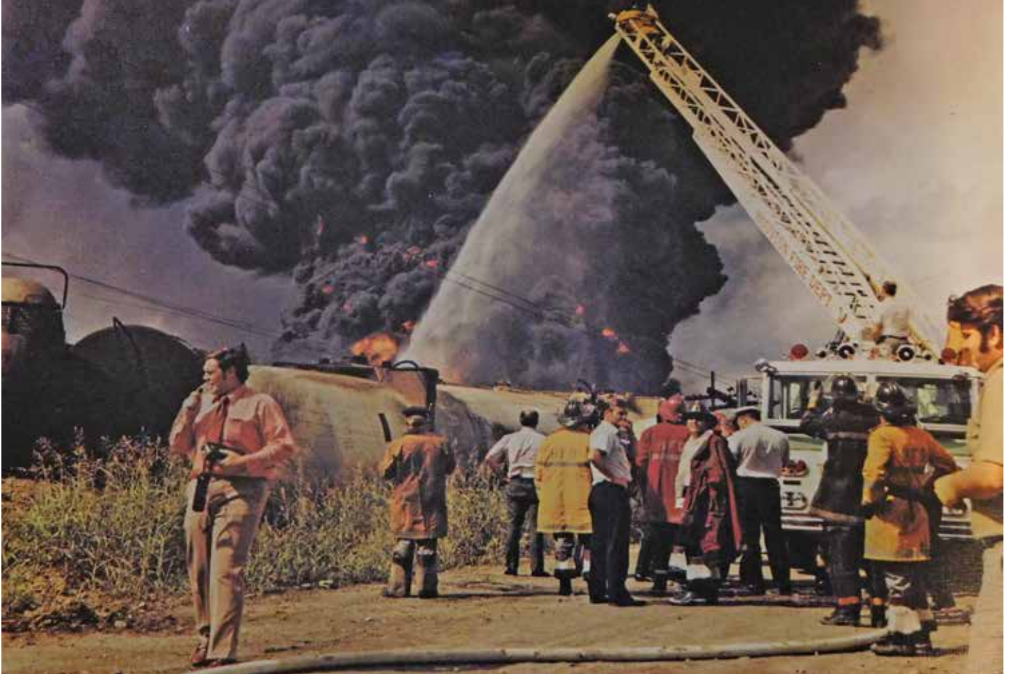
A train carrying vinyl chloride and butadiene derailed causing this 1971 fire on Mykawa Road at Almeda Genoa. A subsequent explosion (boiling liquid vapor explosion or BLEVE) killed one firefighter and injured many of those present, some severely. It also separated HFD member Richard Sadler Jr. from his son and son-in-law, also firefighters, leaving him in despair until he learned they were safe. The fire resulted in formation of the HFD Haz Mat team.
