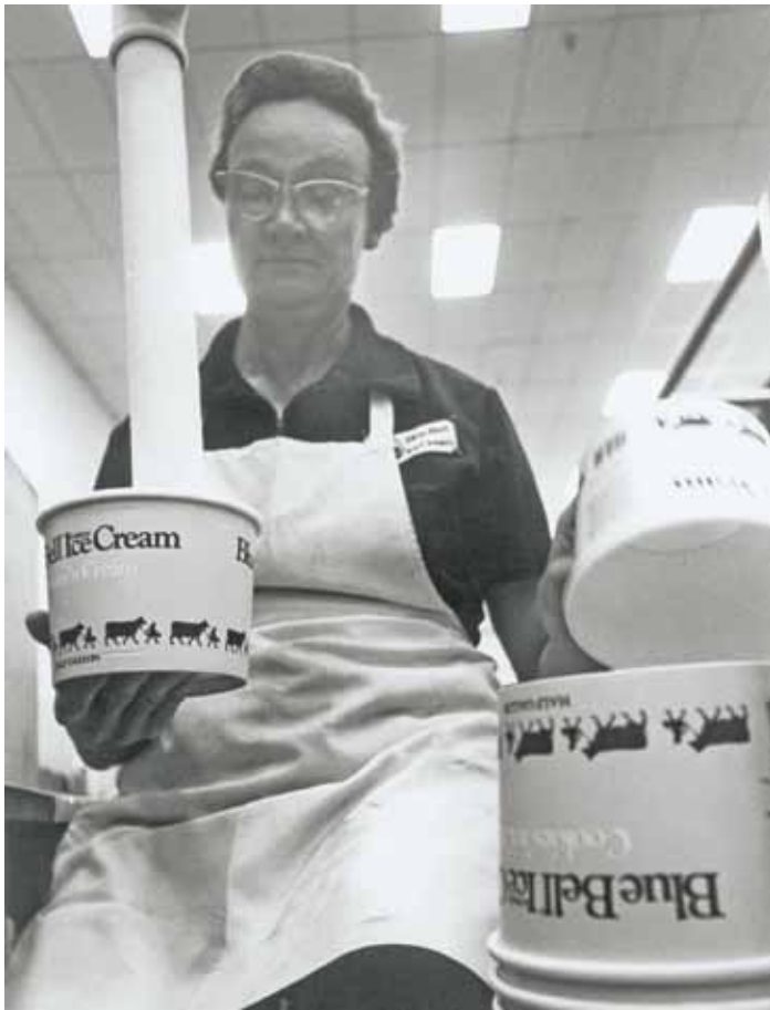
Employees like Lee Dell Krause filled cartons manually for years after the facility made technological improvements. This required “almost a juggling motion as an empty carton was placed under the one being filled by a stream of ice cream.” She then passed the full carton to the next person for sealing and moved the empty carton under the nozzle (all without spilling!).
