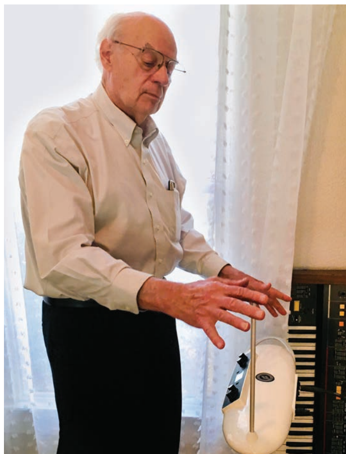
Here Lienhard demonstrates a theremin, a musical instrument that is played not by touching but by moving one's hands to interrupt the magnetic fields to control its volume and pitch. The theremin is discussed in episodes 1818 and 3070 by Andrew Boyd.
